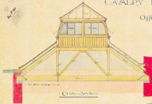
Details of Lantern in Mess-Kitchen
